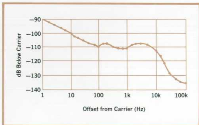
Fig. 3. Typical single-sideband phase noise measured at output of Model 3330A/B Automatic Synthesizer in 1-Hz bandwidth with instrument operating at 12 MHz.
